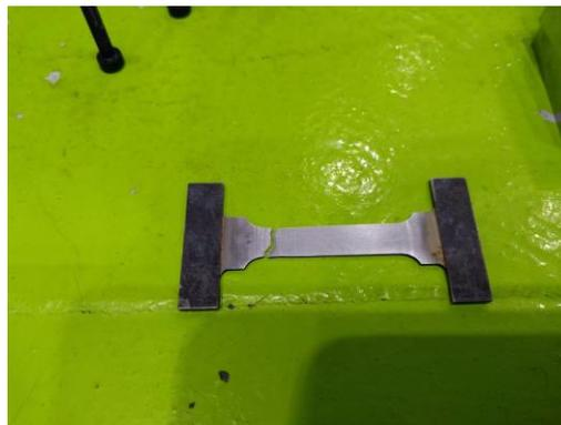
Fig. 4 the fractured sample.
