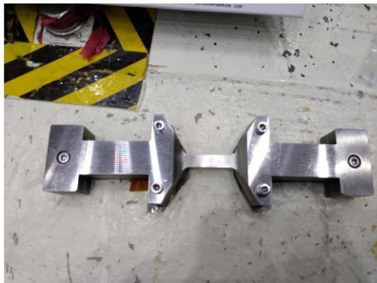
Fig. 2 The sample attached on the anvils.
