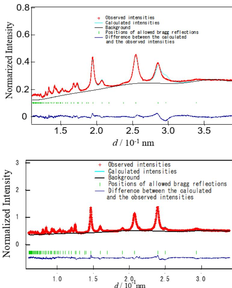
Fig. 1 Rietveld refinement patterns of  $\text{MgCo}_{2-x-y-z}\text{Ni}_x\text{Mn}_y\text{Al}_z\text{O}_4$  in a)  $x=0.25, y=0.25, z=0$ , and b)  $x=0.2, y=1.0, z=0.3$  using neutron diffraction.
