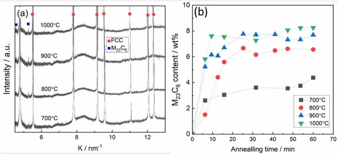
Fig. 6 (a) Fig. 1 Neutron diffraction pattern of the samples after 60 minutes annealing, and (b) an increase of  $M_{23}C_6$  content during annealing at 700°C, 800°C, 900°C and 1000°C.
