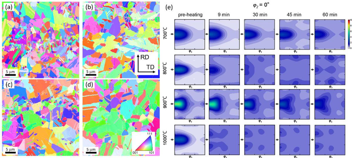
Fig. 3 IPF maps of the samples annealed at (a) 700°C, (b) 800°C, (c) 900°C and (d) 1000°C for 60 mins and (e)  $\phi_2 = 0^\circ$  sections of ODFs calculated from neutron diffraction data of 1%C-doped CoCrFeNi alloy during the annealing.
