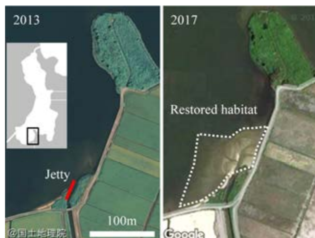
Fig. 3 Restored clam habitat using LKs. Jetty was build up at a river mouth in 2007.
