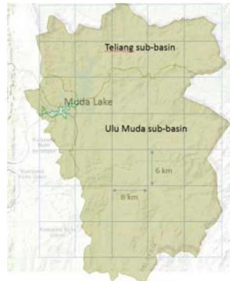
Fig. 2 Catchment model and grid of hydroclimate model
